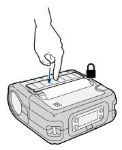
**7** Press and hold the **Feed** button for more than two seconds to calibrate the media.
